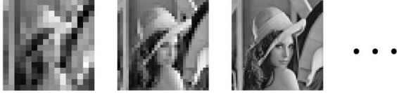
Figure 3: Left is the low resolution residual. The images are obtained by applying the inverse wavelet transform to the wavelet representation of different scales. Moving to the right more detail is added (lower scales) until the final image is obtained.
